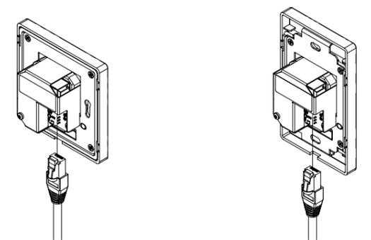
4. Click off the front panel. Screw the Wall-S1 unit into the electrical box. - Put the front panel on - and click it into place.
